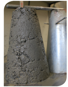
Above - Figure 4: The workability is essential for the market acceptance of new cements. Low slump can be improved with PCE in the cement additive.
