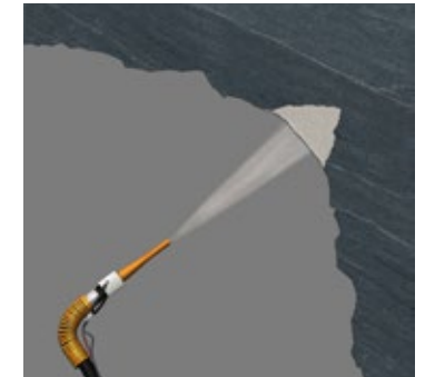
Fig. 7.2: Filling of overbreaks
