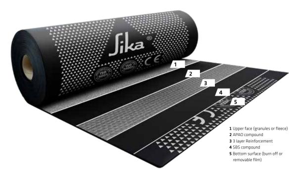
SikaBit® Pro 9 Series bituminous membranes are developed to offer a safe and secure solution for any environment, the SikaBit® Pro Bituminous Membranes range includes detailing materials for completely flamefree Safe2Torch-compliant roof installations.
