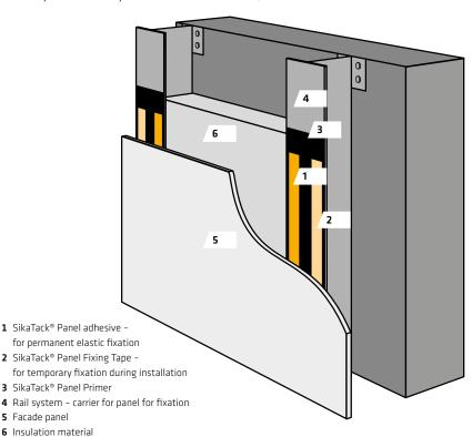
Facade design and installation with SikaTack® Panel System must be done with the support of our technical sales force. Please contact us with your panel cladding project to ensure a beautiful, safe and durable facade.
